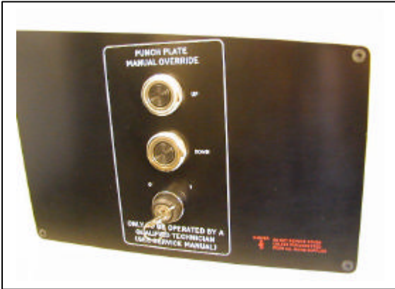
5. Manual setting on control panel.
