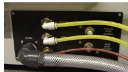
Process Water – Top Yellow Wash Water – Bottom Yellow Waste Water – Clear Braided Air Supply to Pump – Red
